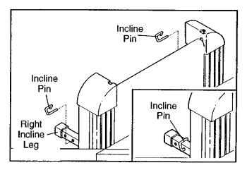
Adjust the left incline leg in the same way. Make sure that both incline pins are inserted from the direction shown.
